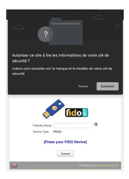
After pressing the key, the FIDO device is enrolled and can be used to log in on systems requiring FIDO authentication.
