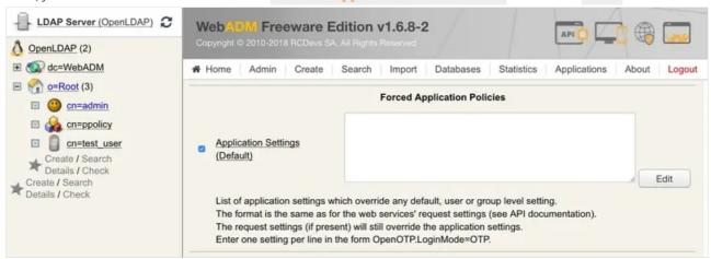
In the Applications box on the top left, click on OpenOTP and now, you are able to reconfigure completely the OpenOTP application for pfSense. But here, only one setting interest us who is the Challenge Mode Supported. You have to set the setting to No because OpenVPN doesn't manage the RADIUS Challenge. Of course, my default configuration of OpenOTP is set for LDAPOTP login mode.
